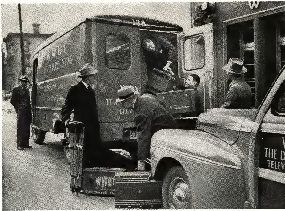
Remote crew of Detroit News tele station, WWDT, loading cameras in the two-car mobile unit. Station wagon (nose, right) carries crew and associated equipment.
